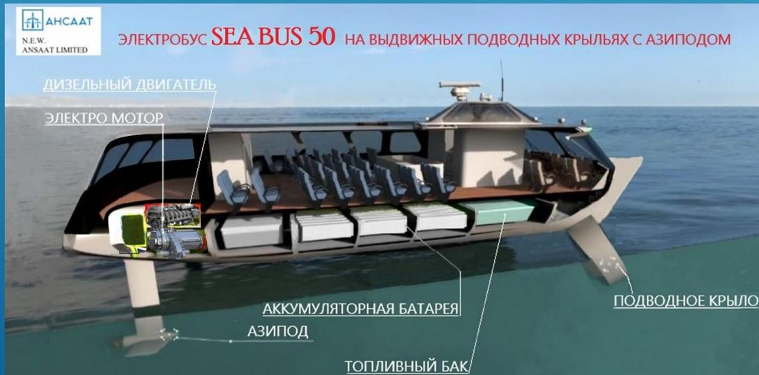
OUTBOARD ELECTRIC MOTOR AND INTERNAL COMBUSTION ENGINE
